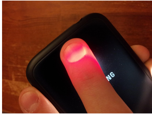
Fig. 1. How to place the finger while measuring heart rate
